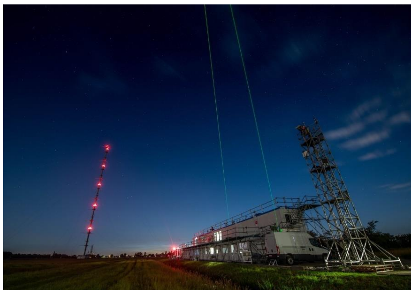
Figure 5.17. Lidar instruments in operation during CINDI-3 at the Cabauw Atmospheric Research Station. The two green beams originate from Caeli and EMORAL.
