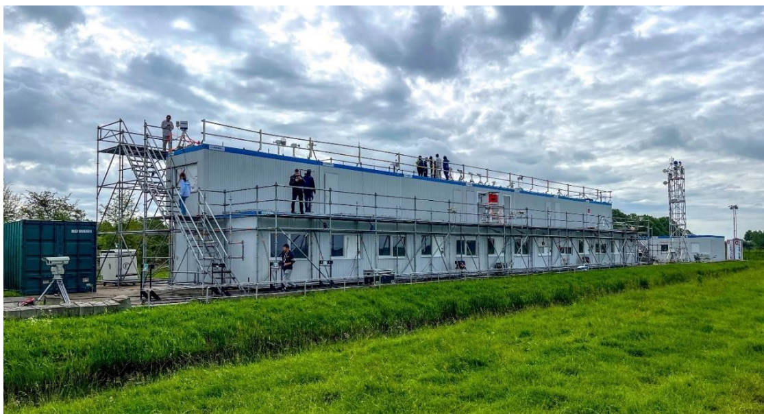
Figure 2.4. CINDI-3 two-storey container setup with scaffolding at the remote sensing site. One of the two LP instruments can be seen next to the containers (on the left side of the picture).
