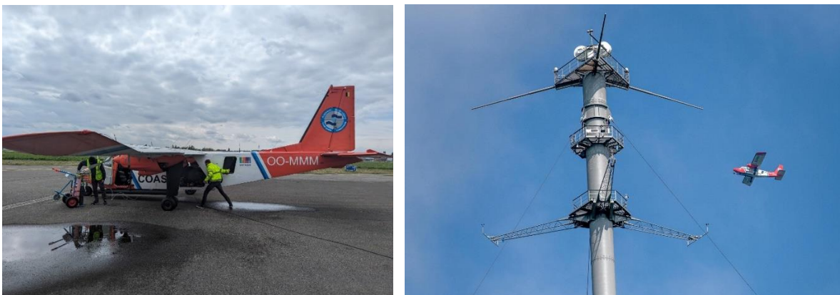
Figure 5.36. Left: The BN-2 Belgian Coast Guard Aircraft 'OO-MMM' during instrument calibration at the Antwerp airport. Right: Same aircraft during a spiral flight centered on the KNMI measurement tower at Cabauw.
