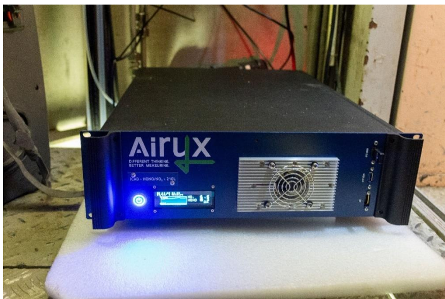
Figure 5.2. ICAD in situ instrument for \text{NO}_2 and HONO placed inside the tower at the first platform at 27 m above ground level.
