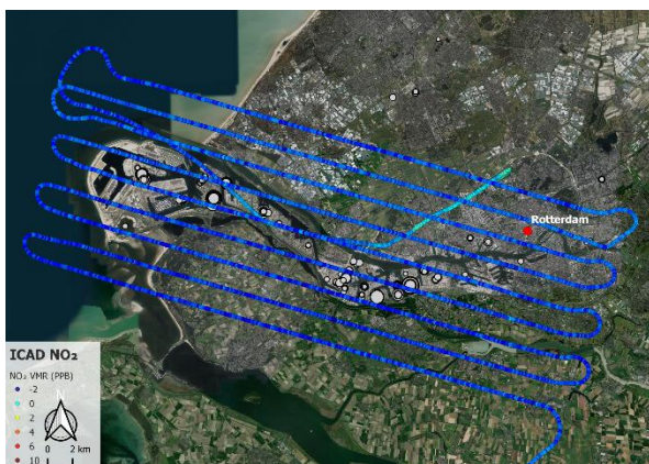
Figure 5.40. Distribution and concentrations of NO 2 VCDs in the industrial and urban area of Rotterdam and over Cabauw, as observed by SWING+ on 7 June 2024.
