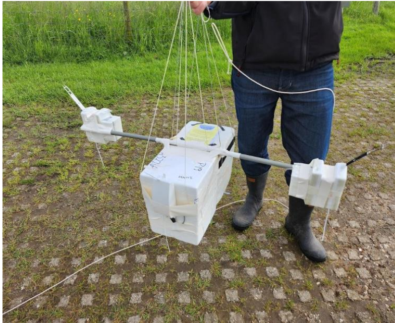
Figure 5.15. Balloon payload consisting of a combined NO 2 and ozone sonde interfaced with one Vaisala RS41-SGP radiosonde and 2 Weathex NO 2 sensors both interfaced with individual Weathex WxR-301D radiosondes.
