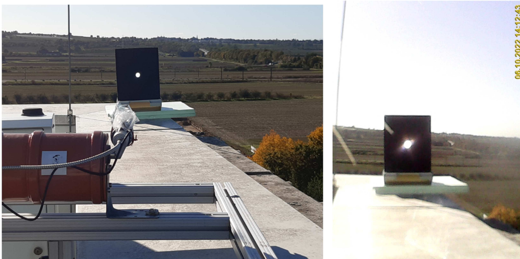
Fig. 6 Left: Measurement set up for the determination of the location of the viewing direction within the image of the telescope camera. A light source in front of a black screen is placed in the field of view of the instrument. Right: image of the telescope camera after the telescope was turned into the direction for which the highest light intensity is received. The location of the light source in that image indicates the viewing direction of the telescope.
