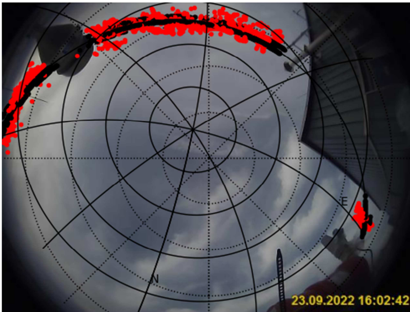
Fig. 5 Example of the determination of the exact location of the zenith direction within the fish-eye camera image for the Mainz instrument. The correct coordinate system was determined by fitting the calculated trace of the sun position (thick black line) to the observed sun positions (red dots). 5 camera-parameters (3 angles, translation, and scale) were fitted to match the observations. The dotted contours show the original coordinates, the solid contours the fitted coordinates. The center indicates the exact zenith direction. The calibration was performed by Ankie Pieters, KNMI.
