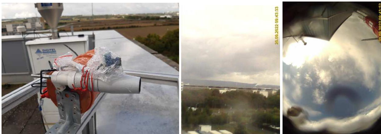
Fig. 4 Left: Mounting of the telescope camera at the Tube MAX-DOAS instrument on the roof of the MPI for Chemistry in Mainz on 20.09.2022, 09:43 UTC. On this day it was occasionally raining. Center and right: camera images from the telescope camera and fish-eye camera, respectively, taken at the same time. Although some blurring is caused by the water drops on the foil, the sky conditions can be characterised.
