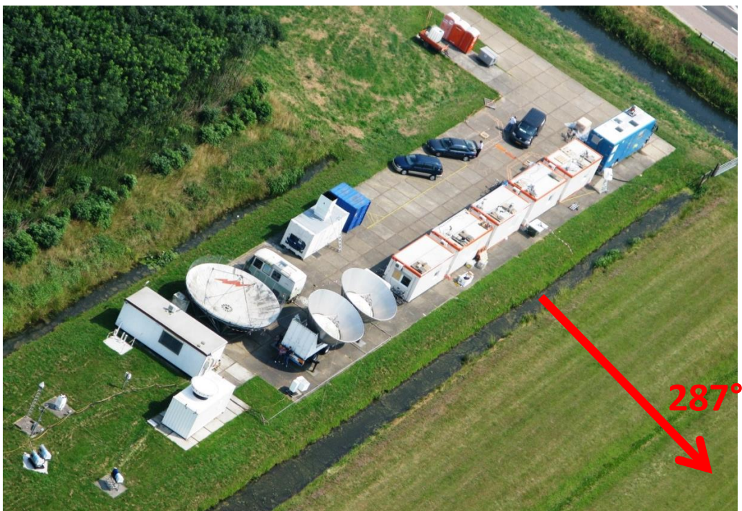
Figure 8: Aerial picture of the CESAR remote-sensing site, as configured during the CINDI-1 campaign in 2009. DOAS and MAXDOAS systems were installed on the roof or in front of the 5 white containers.
