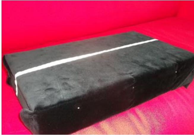
Figure 12: Black target with a white stripe prepared for elevation calibration during the CINDI-2 campaign (© M. Gu and T. Wagner/MPIC-Mainz).
